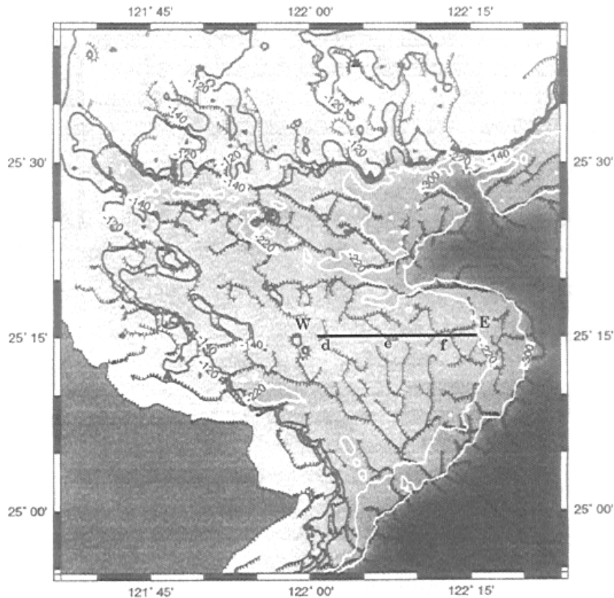
Fig. 5. Map showing 120, 140, 220 and 300m isobaths indicating the traces of the inner and the outer shelf breaks. The E-W straight line is the location trace of the seismic profile shown in Figure 9. d, e and f mark the targets found along the profile intersecting with the "break" lines. The "break" lines are done by the self-developed automatic line extraction computer program (Chang, 1997). These "break" lines indicate the edge traces of the break topography as discussed in the text.
